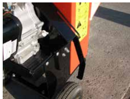
Figure 3.2, Operating Position Belt Engaged
