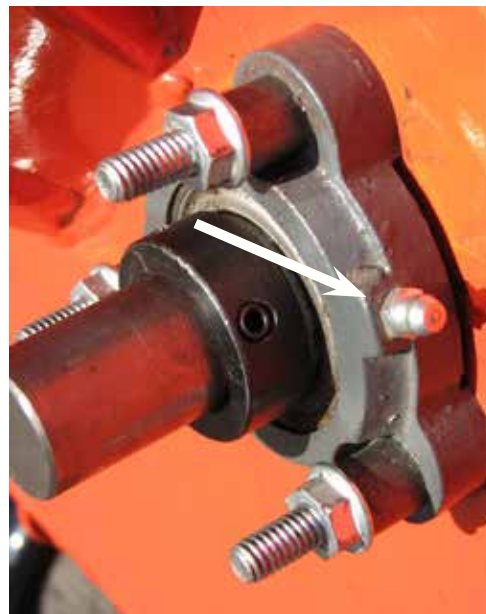
Figure 5.13, Chute Side Bearing Zerk
