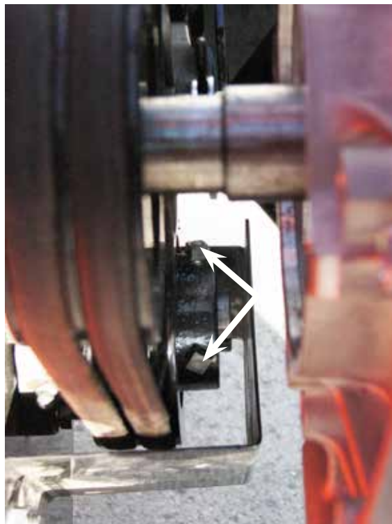
Figure 5.10, Engine Side Bearing Set Screws
