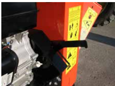
Figure 3.1, Start Position Belt Disengaged
